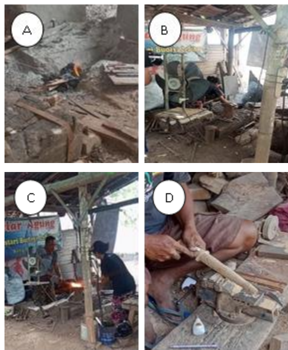
Figure 2. Process flow for making a Keris Madura (A. Preparation, B. Forging, C. Technical work, D. Final work)
